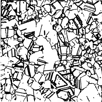
FIGURE 392. Metallographic structures of annealed cartridge brass (70% Cu — 30% Zn), grain size 0.050–0.055 mm. Etched with \text{NH}_4\text{OH} + \text{H}_2\text{O}_2 . \times 75 . (Left) Light etch. (Right) Contrast etch.
